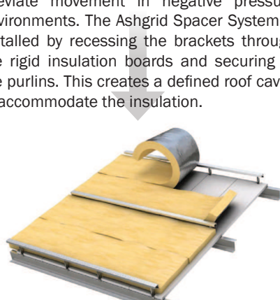
Fig b: Bulk insulation to the required depth can then be installed over the installed rigid boards. Care needs to be taken that the bulk insulation is packed tightly to avoid thermal bridging. It is recommended practice to stagger the joints of the insulation when more than one layer is installed. It is imperative that a vapour barrier be installed in high condensation regions.
